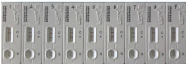
1: 阴性对照; 2: 5.1 \times 10^7 cfu/mL; 3: 5.1 \times 10^6 cfu/mL; 4: 5.1 \times 10^5 cfu/mL; 5: 5.1 \times 10^4 cfu/mL; 6: 5.1 \times 10^3 cfu/mL; 7: 5.1 \times 10^2 cfu/mL; 8: 5.1 \times 10^1 cfu/mL; 9: 5.1 \times 10^0 cfu/mL 1: Negative control; 2: 5.1 \times 10^7 cfu/mL; 3: 5.1 \times 10^6 cfu/mL; 4: 5.1 \times 10^5 cfu/mL; 5: 5.1 \times 10^4 cfu/mL; 6: 5.1 \times 10^3 cfu/mL; 7: 5.1 \times 10^2 cfu/mL; 8: 5.1 \times 10^1 cfu/mL; 9: 5.1 \times 10^0 cfu/mL
