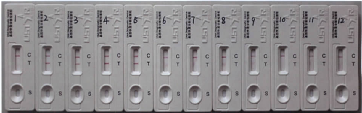
1: 阴性对照; 2: 副溶血性弧菌 ATCC 17802; 3-4: 副溶血性弧菌 分离菌株; 5: 宋氏志贺氏菌 CMCC (B) 51592; 6: 肠炎沙门氏菌 ATCC 13067; 7: 单核细胞增生李斯特氏菌 ATCC 7644; 8: 小肠结肠炎耶尔森氏菌 CMCC (B) 52207; 9: 大肠埃希氏菌 ATCC 25922; 10: 弗氏柠檬酸杆菌 ATCC 43864; 11: 产酸克雷伯氏菌 ATCC 43165; 12: 阴沟肠杆菌 ATCC 700323 Note: 1: Negative control; 2: V. parahaemolyticus ATCC 17802; 3-4: V. parahaemolyticus isolates; 5: S. sonnei CMCC (B) 51592; 6: S. enteritidis ATCC 13067; 7: L. monocytogenes ATCC 7644; 8: Y. enterocolitica CMCC (B) 52207; 9: E. coli ATCC 25922; 10: C. freundii ATCC 43864; 11: K. oxytoca ATCC 43165; 12: E. cloacae ATCC 700323
